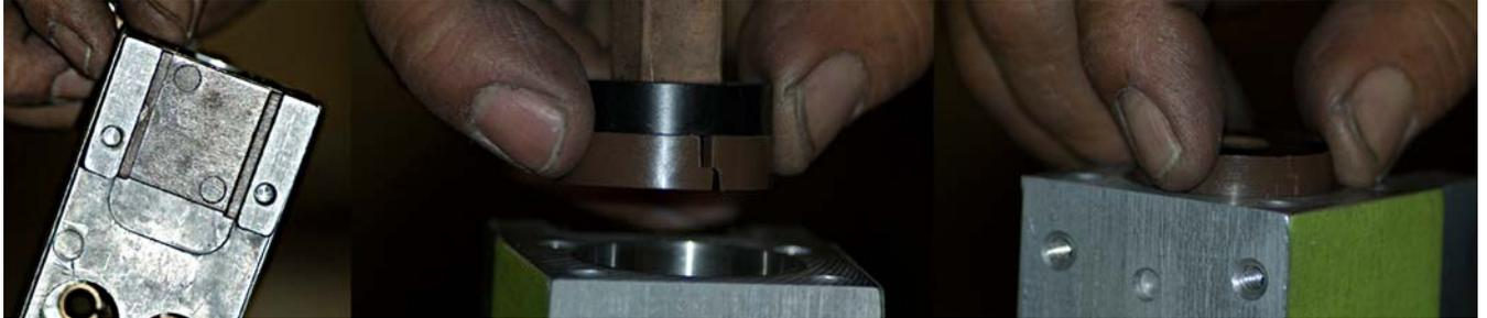
2 Place block upside down, so you can look through two large holes on bottom of casting. These are where the 1210-1 & 1209 shaft will go. Use both thumbs, to tilt piston so gear teeth are at an angle. 1210-1 gear goes in, furthest away from your body. Use thumbs to twist piston gear rack into place. Drop 1209 in the bottom space or closest space towards you. Tilt the 1211, until the 1209 gear drops down. A few taps with a hammer might be necessary.
