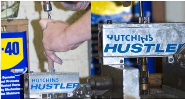
Place the 1215 Block on top of the two aluminum blocks. With a hammer and bit, tap out the 1209 and 1210-1 gears through the top of the valve plate. They should drop through the bottom of the block.
