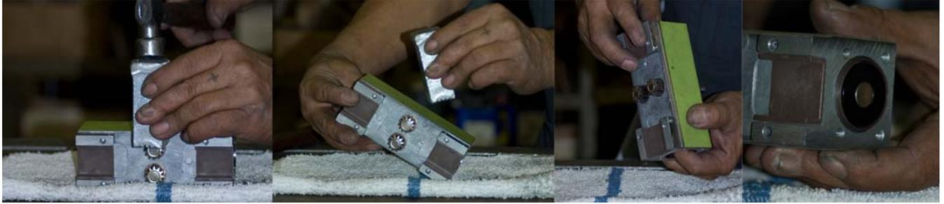
5. Use Spray gasket glue or Silicone Sealant on 1214 Valve Plate. When tacky, place on motor block with 1225 timing plate towards front.
