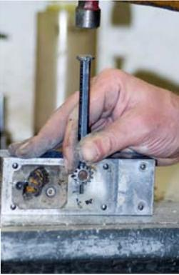
Use a 1/8 drift punch to push the 1252 pin out of the 1227 gear. Push pin out just enough to free 1210-1 gear
