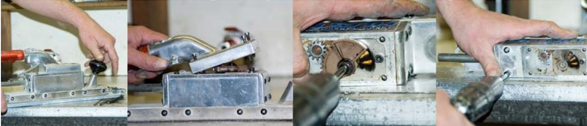
Remove 1235S Side Rails and the 1204 Drive Shoe will come off now. This part should be replaced when you have gouges in the metal on the outer edge (see picture below). The counterweight bar 1242 will come out now. The Old style bar will not have the counterweight spring.
