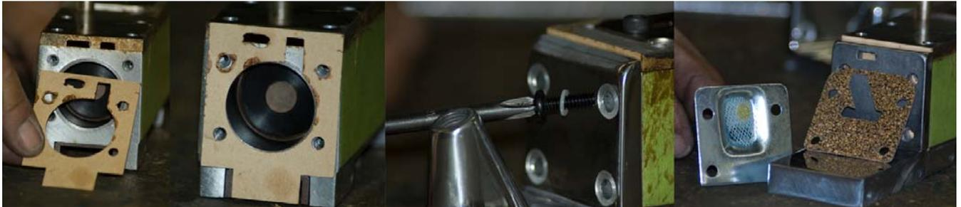
7. We will now install the 1227 gear on top. With front to you left and rear to right line up hole in 1210-1. Line up 1227 gear hole with hole in shaft. Press 1227 gear down with press, or gently tap down with hammer. Now use 1252 to secure gear. You will need to put tool on side to do this. Use a 1/8 punch to press pin all the way into gear. Turn the gear you just installed counterclockwise till it stops.
