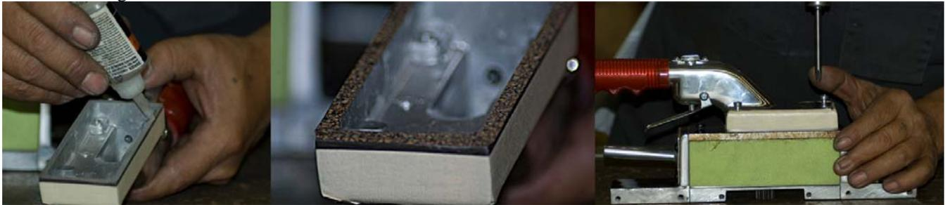
10.Clean any excess glue off. Turn over tool and check gears to make sure they spin freely. Prepare to install 1242 counterweight bar. Install 4-1207S ware strips. Press in with holes towards center gears. Glue the sponges on. The thin sponge in front, Thick sponge in rear.
