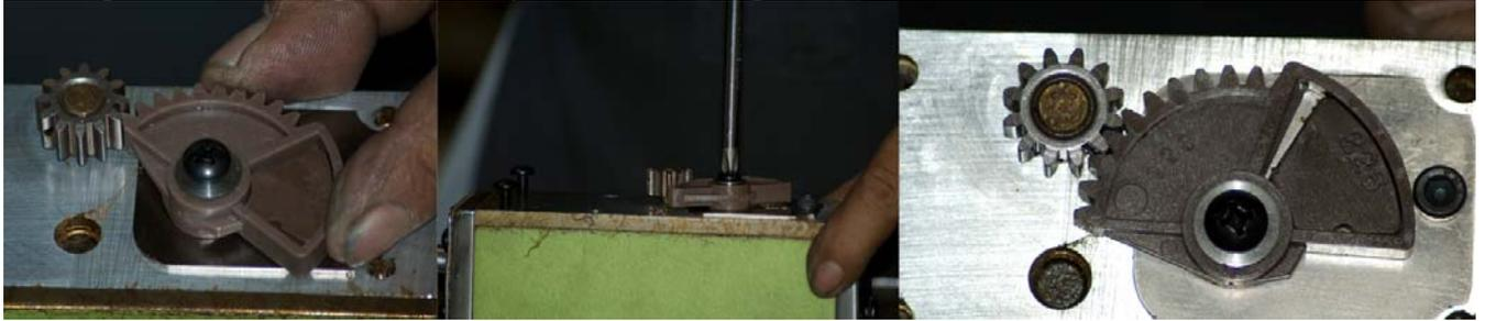
9.Attach new 1232 gasket to 1233 handle. Glue gasket on one side. Wait till tacky, then press down onto 1233 handle. Please give a few hours for handle to dry, unless using minute glue. After drying time, Attach handle housing with screws.
