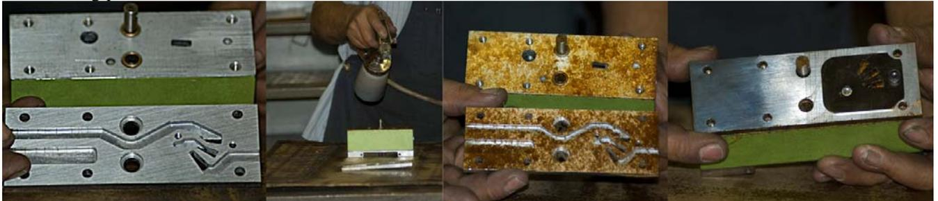
6. Use new 1212S gaskets and glue onto each end of motor block. Make sure to put gasket on, so airway is not blocked. The center hole has a notch. Align that towards the top of the tool. Attach 1217 front with screws, and small clear washers. Hand tighten screws, then tighten with screw gun. The 1218 rear can then be attached in the following order: 1220 gasket, 1218 rear, 1222 gasket, & 1223 muffler. Screws with no washers are used.
