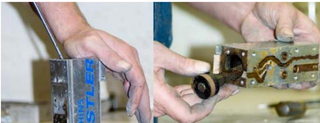
Pry off the 1214 Valve plate. The 1211 Piston and 1212S Piston Rings with ends will now come out. Rings should have no wear, and have a good seal. It is usually a good idea to replace these with each repair, unless the tool is very new.
