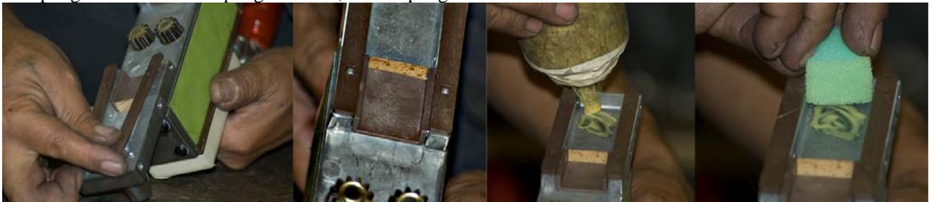
11.Hold tool in hand angling handle towards you body. Turn Right gear (1210-1 long gear) all the way counterclockwise till it stops. Put counterweight bar 1242 in, lining up spring first. The second tooth on counterweight bar will line up towards rear of tool.
