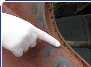
BEFORE: Rusted, leaking seam.
