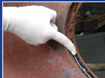
Press and contour bead into seam.
